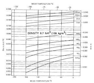
Effect of interstitial gas pressure and temperature on thermal conductivity of 8.7 lb/ft<sup>3</sup> (139 kg/m<sup>3</sup>) expanded, evacuated perlite insulation.
