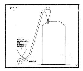
One low-positive-pressure system (Fig. 3) employs a venturi to draw the perlite into the stream of air coming out of a blower. Often a cyclone is used on top of the tank. No air lock is required because the cyclone is under pressure.
