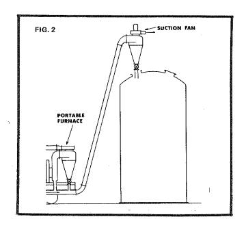
To avoid the question of the danger of collapsing the tank, a cyclone can be erected on top of the tank (Fig. 2), with a draft fan to create suction and an air lock to discharge the material into the tank. This is a low-pressure-differential system. A cyclone can also be used on low-positive-pressure systems to obtain better collection efficiency than might be obtained by settling alone.
