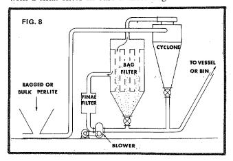
The high-pressure, low-gas-volume methods have the advantage of permitting the use of reasonable quantities of dried air, dry nitrogen, or any other gas which may be specified. They also allow more precise deposition of the perlite.
