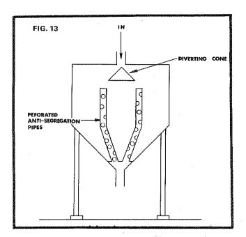
of the silo. A silo equipped with perforated pipe antisegregation facilities is shown (Fig. 13).
